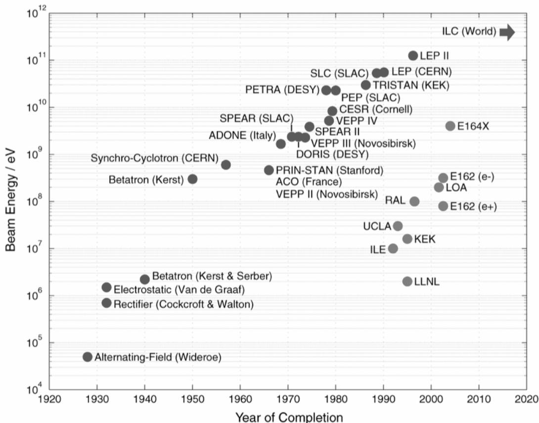
**Figure 1.** The Livingston plot showing the energies of RD (dark gray) and plasma (light gray) acceleration techniques. Energies obtainable in plasma acceleration experiments have risen rapidly over the last decade and may soon surpass energies achievable with RF technology [4].
