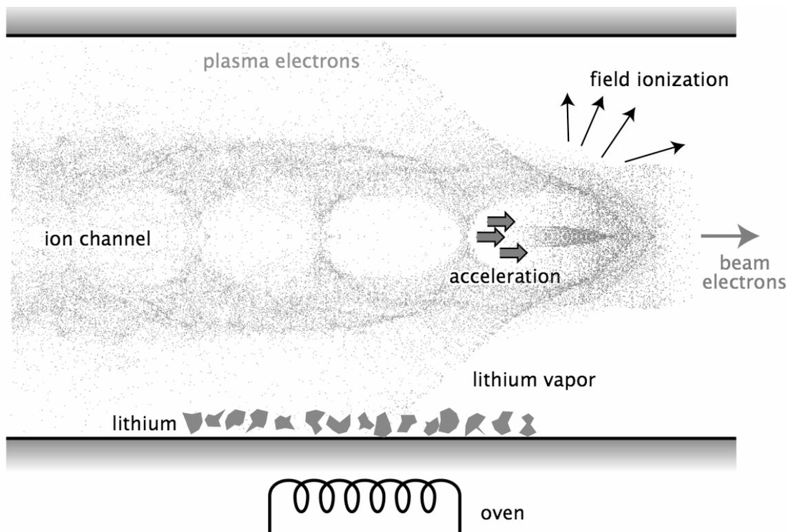
**Figure 2.** Wakefield formation—a drive pulse expels plasma electrons, creating a column of positive ions; plasma electrons oscillations create ‘buckets’ containing large electric fields that can be used for particle acceleration [4].
