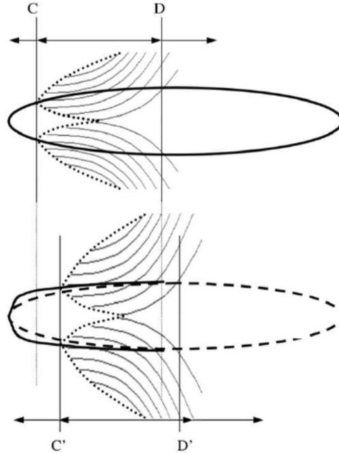
**Figure 4.** Self-ionization, in which the plasma medium is ionized and the wakefield is created by a single drive pulse. The ionization front, labeled D above, is the plane in which the entire transverse profile of the drive beam lies within the ion column. The portion of the beam ahead of the ion front is eroded, and the ionization front moves toward the rear of the drive pulse.
