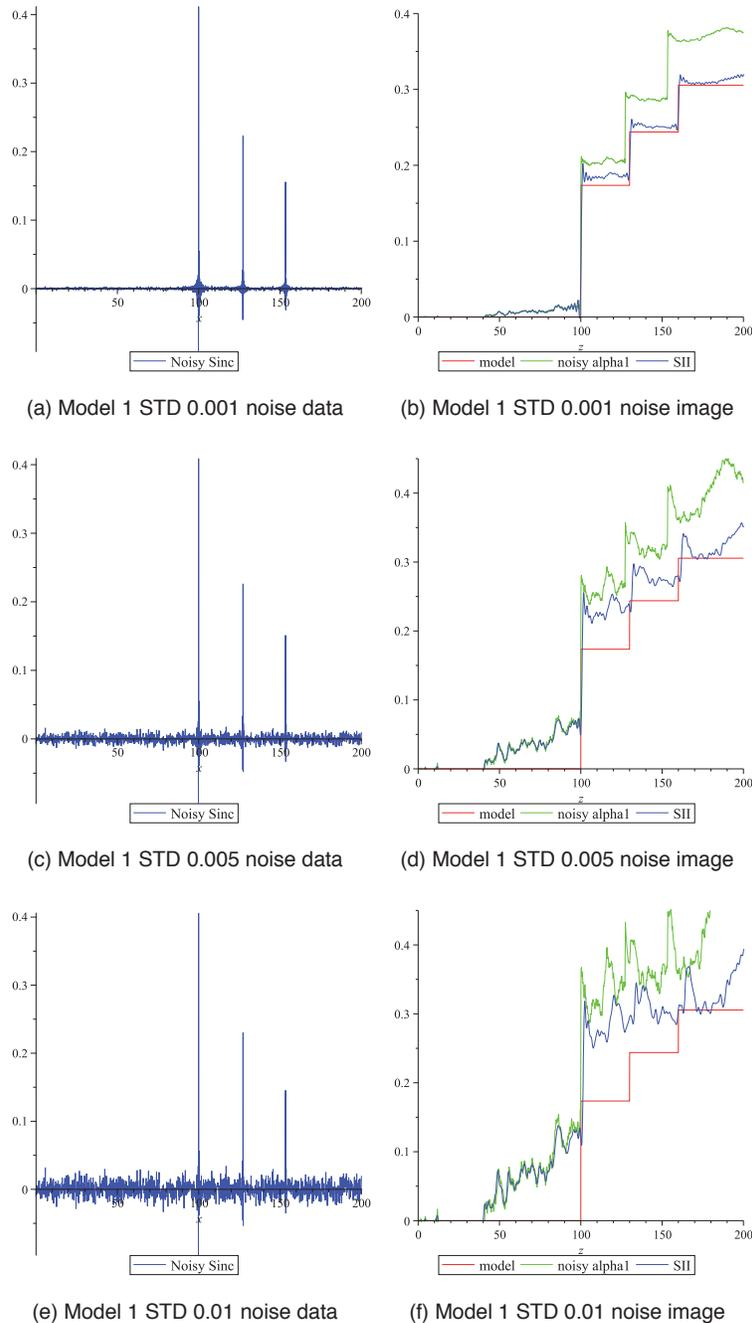
**Figure 2.** Model 1 imaging algorithm with increasingly more noise
