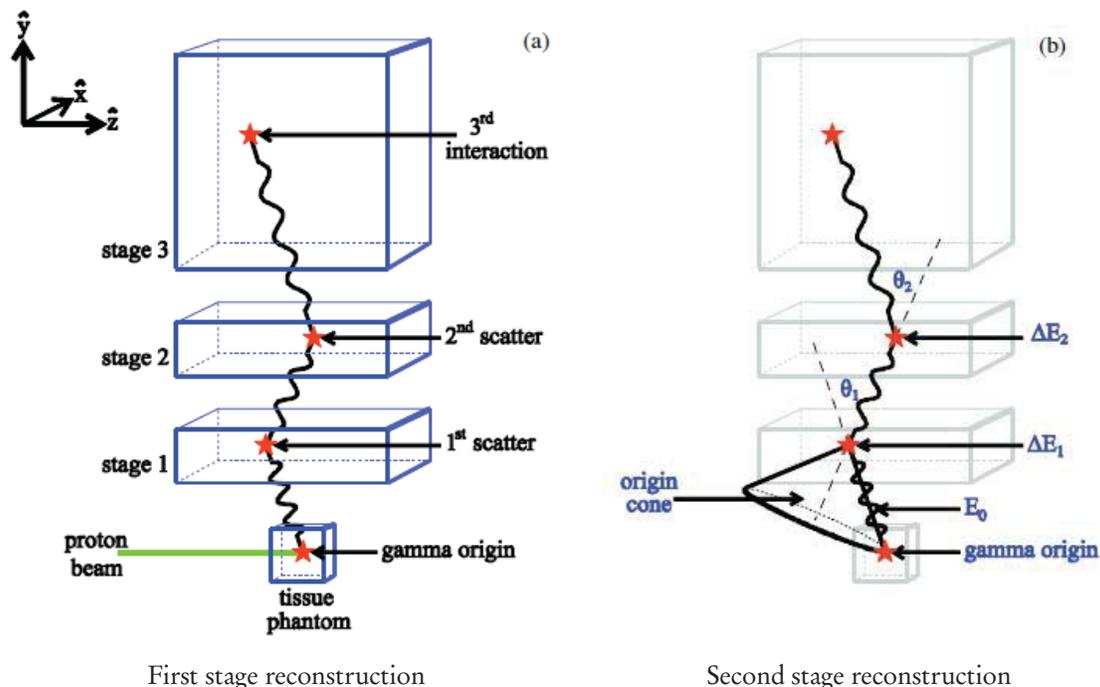
Figure 1. Gamma ray scatter and its image reconstruction.
